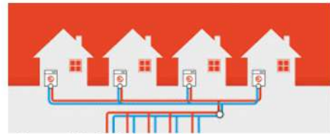
FIGURE 10: GSHP SUPPLYING A SMALL CLUSTER OF DOMESTIC PROPERTIES (SOURCE: KENSA HEAT PUMPS)
